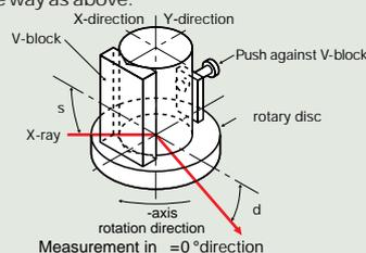
**Case 3: Obtain a deviation of a crystal axis relative to a pasted plate which acts as the physical reference.**
