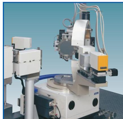
Bond method attachment mounted on ATX-E
