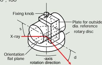
**Case 5: Obtain an angular deviation on a lattice plane relative to a wafer (the wafer surface acts as the physical reference):**
