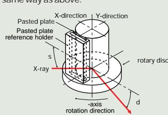
**Case 4: Obtain an angular deviation on the lattice plane relative to the orientation flat (OF) of the sample. (the sample flat acts as the physical reference):**
