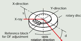
**Case 6: Obtaining an angular deviation of a lattice plane relative to an orientation flat (OF) of a wafer (the sample flat acts as the physical reference):**
