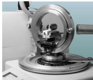
**2-Axis Adjusting Ingot Jig for Determination of Cutting Orientation :**
