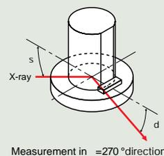
**Case 2: Obtain a deviation of a crystal axis relative to the outer circumference of the sample which acts as the physical reference.**
