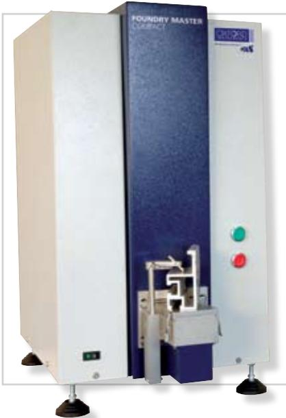
Optical Emission Spectroscopy (OES) has for many years been the most accurate and reliable technique for producing qualitative and quantitative analysis of materials composition. It works by exciting atoms with energy that comes from a spark formed between the sample and electrode. The energy of the spark causes the electrons in the sample to emit light which is converted into a spectral pattern. By measuring the intensity of the peaks in this spectrum, Oxford Instruments' OES analysers can
